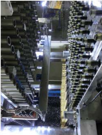
Looking down from the take out plate to the cold half (figure: MHT)
